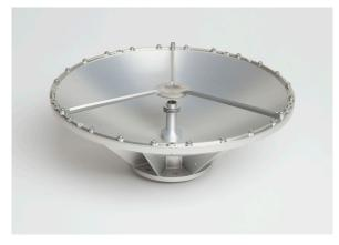
PIM is prevented via a high pressure flange between the septum polarizer and the reflector. The standard antenna is circularly polarized (RHCP or LHCP), with the unused port of the septum polarizer terminated. The design can easily be changed to dual polarization operation by adjusting the septum polarizer design only.
