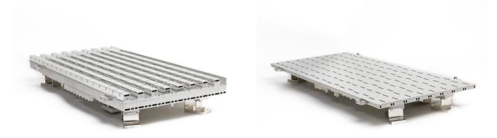
A breadboard of the scatterometer antenna is used by the NOAA's famous hurricane hunter aircraft "Miss Piggy" to improve wind velocity measurements.
